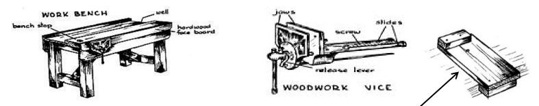
**Bench Hook**- used for holding the timber while you saw or chisel on the bench and at the same time preventing the bench top from damage.
