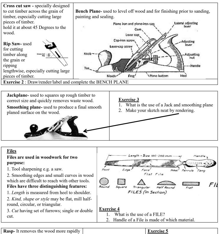
**Rasp-** It removes the wood more rapidly than a file but leaves a coarse finish, which must be smoothed with a file or glass paper.
