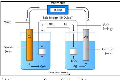
Anode reaction (oxidation): Cathode reaction (reduction):
