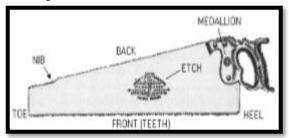
(iv) Rip Cut Saw: cut parallel to the direction of the wood grain.
