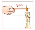
Conduction transfers heat within a body or between two bodies that are touching. It is a point-by-point process of heat transfer. Conduction occurs in solids, liquids, or gases that are at rest.
