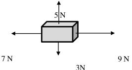
Determine the magnitude of the resultant force acting on the block. (first work out the resultant from the opposite vectors, ie right and left, then up and down, then add this two using vector addition, join start to end, calculate the length of this line using Pythagoras theorem.
