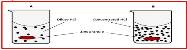
This illustration shows that zinc granules (of same size) being placed in two different beakers of HCl solutions (dilute and concentrated solutions).
