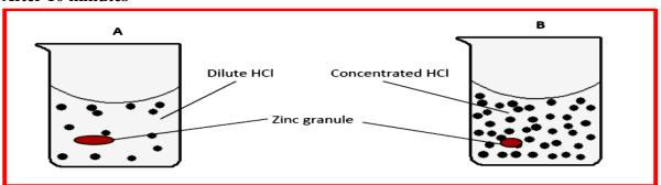
The illustration above shows that zinc granule reacted faster in conc. HCl than in the same volume of dilute HCl at a given time. This is because the concentrated HCl had more reacting particles to collide with zinc granule, thus more chances of effective collision, which increased the rate of the reaction.
