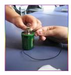
With one end of the piece of wire, the pupils wrapped this around the base of the bulb; then they touched the bottom of the bulb to the centre of the terminal of the battery. If they touch the other end of the wire to the bottom of the cell, the light should go on because a current of electricity is flowing from the cell to the bulb. The path the current takes is called an electrical circuit. If there is a break in this current, the current stops, and the light goes out.
