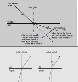
Figure 7.11: Light moving from one medium to another bends towards or away from the surface normal. The angle of refraction  $\theta$  is shown.
