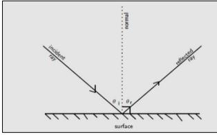
The angles of incidence and reflection are measured with respect to the surface normal.
