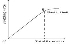
If the elastic limit is not exceeded, F  $\alpha$  x. Thus the spring follows Hooke's law given by:
