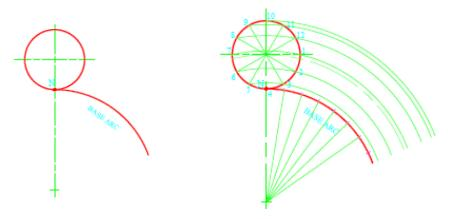
Step 3: Extend the lines from the centre of the base arc to the centre arc to locate C1, C2, etc. Set the compass to the radius of the generating circle and with centers as C1, C2, C3, etc, inscribe arcs on the arcs drawn from each point of the generating circle in its rolling direction.
