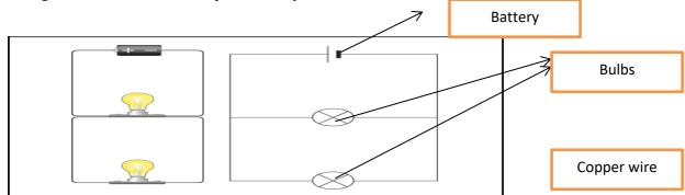
In a parallel circuit, if one bulb gets bad the other one will light because they have 2 different pathways for the current to flow. And if you add more bulbs in parallel circuit it will be bright.
