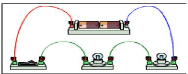
The components are connected end-to-end, one after the other. They make a simple loop for the current to flow round. You can connect several bulbs in series. When the switch is open, no current can flow. When the switch is closed, the circuit is complete and the current flows. **The more bulbs the dimmer the light will be. If one bulb is bad the whole circuit will not function**.
