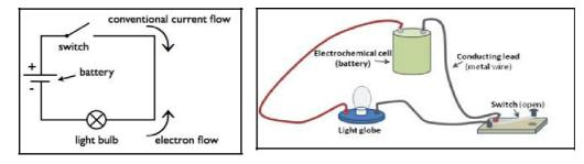
This is the simple complete circuit: Connect the bulb to the battery; the electricity will flow from battery through the copper wire to the bulb and the bulb will light.
