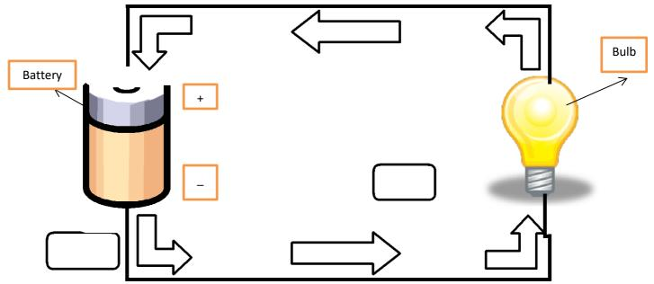
The electricity flows from the **negative terminal of the battery**, through the bulb and back **to the positive terminal** of the battery.
