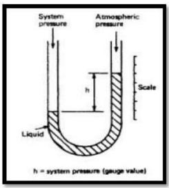
Measuring gas pressure by using manometer
