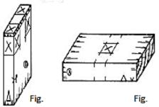
(d) Use the same setting to mark both faces of piece A and use a try square and (already smoothed) piece B to mark the remaining two lines for the width of the mortise (Fig. 5). Mark the waste with a small cross.
