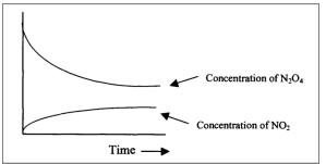
In the initial state, only  $N_2O_4$  is present in the vessel and there is no  $NO_2$ .
