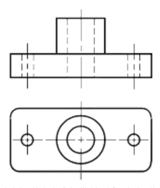
**Given:** The sketch, plan and the elevation of a shaped block drawn in first angle orthographic projection and the cutting plane line **B-B**
