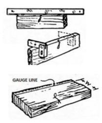
gauge lines. Test for straightness and square-ness.
