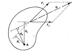
Moment of a force, with respect to a given point, in the same plane, is the product of the force and the perpendicular distance from the point to the line of action of the force. The unit of a moment of a force is the newton metre (Nm) and multiples of this unit i.e. kilonewton metre (KNm), etc.
