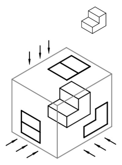
**Note:** When the box is opened, the plan and the end elevation are in line with the front elevation. The plan is drawn in line & above the front elevation and the end elevation drawn in line but on the side of the front elevation where it is viewed from.
