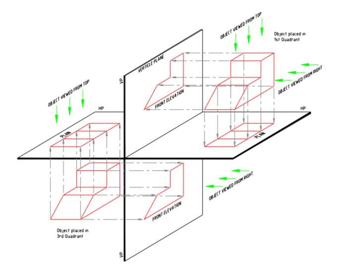
In the first angle projection, the object is viewed from one side and drawn on the other side as is the case with X-rays in the hospitals. While in the third angle projection, the object is viewed and drawn on the same side as is the case with the photos taken from a camera.
