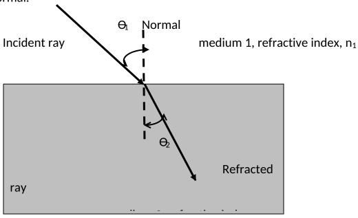
$\Theta_{\!\scriptscriptstyle 1}$  is the angle of incidence,  $\Theta_{\!\scriptscriptstyle 2}$  is the angle of refraction
