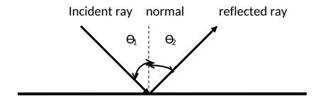
$\Theta_1$  is the angle of incidence,  $\Theta_2$  is the angle of reflection and always measured from the normal.
