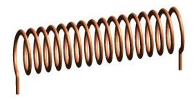
If a current flows in the coil of wire it also behaves like a magnet. This type of magnet is called the electromagnet.
