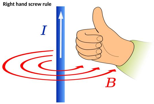
The thumb points in the direction of current and the fingers curl around in the direction of field.
