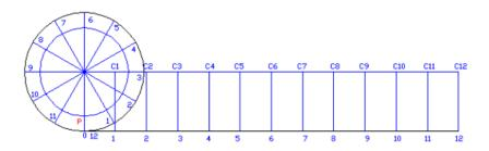
Draw the height lines for the **Inferior Trochoid**, and this is where things are a little different from the construction of a Cycloid.
