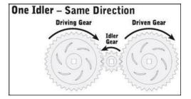
An idler gear is a gear wheel that is inserted between two or more other gear wheels.
