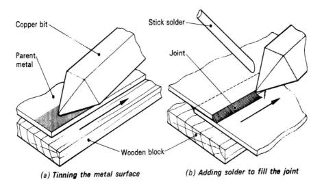
Soldering irons have copper bits because copper has an attraction for
