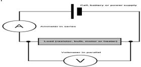
When you make up the circuit connect the cell, load (resistor etc.) and the ammeter first. When this is correct **THEN** connect the voltmeter across the load.
