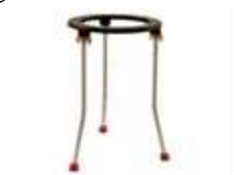
Tripod Stand Used to support flasks and Beakers
