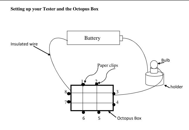
The bulb will light because there is a complete pathway made for electricity to pass through when the two ends of the wire are joined by numbers 3 and 8.
